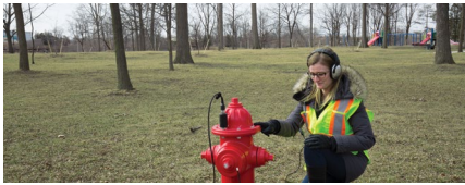
STEP 1: ATTACH SENSOR TO EXISTING PIPE CONTACT POINTS
