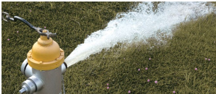
STEP 2: INDUCE NOISE INTO THE PIPE
